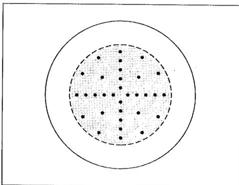
Figure 3: Layout of 32 preselected points for the counting at 3000X.
