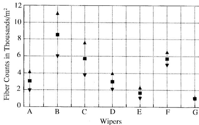
Figure 4. Fiber release comparison (showing high-low ranges) from wipers A—G, as determined by optical microscopy at 20X magnification.
