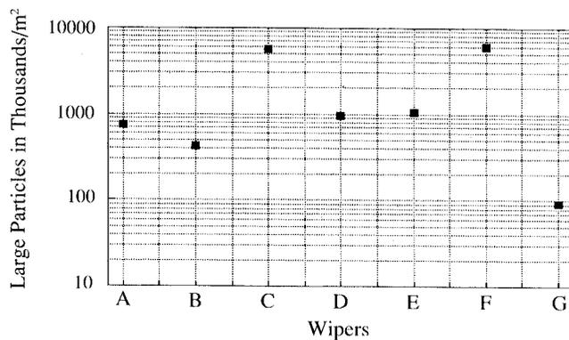
Figure 5. Semilog plot of average values of large particle counts for wipers A—G, as determined by scanning electron microscopy at a magnification of 200X.
