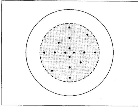
Figure 2. Layout of 16 preselected points for the counting at 200X.
