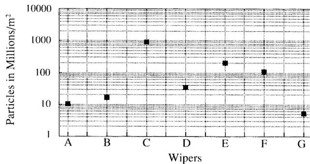
Figure 6. Semilog plot of average values of small particle counts for wipers A—G, as determined by scanning electron microscopy at a magnification of 3000X.
